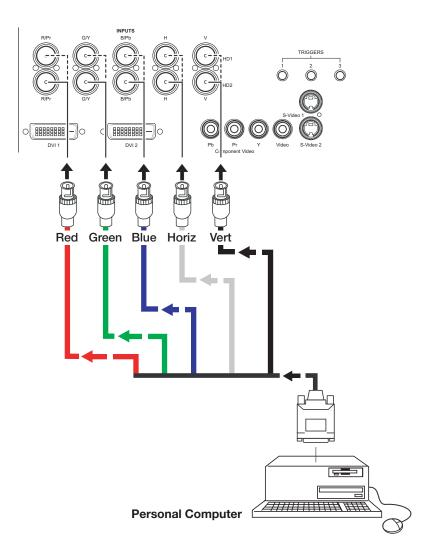
Figure 3-7. Analog RGB Connections
